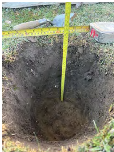
Plate 4: Sample Test Pit Profile Lots 1-2-3; looking west
